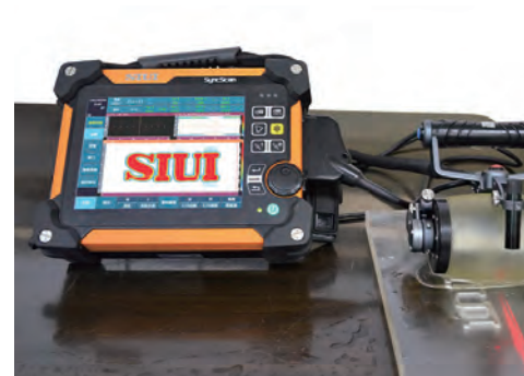
C-Scan in-amplitude on flat pannel engraved with SIUI logo
