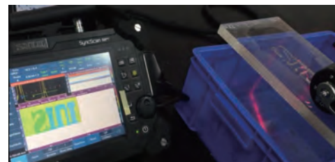
C-Scan in-depth on flat pannel engraved with SIUI logo
